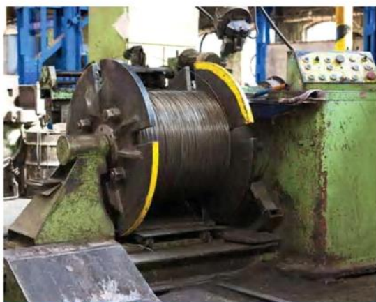
tažný stroj COILS I. – 1000 kg svitky drawing machine COILS I. 1000 kg coils
